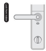
Turn the knob to double-lock. In this case, it is not available to unlock from outdoor.
