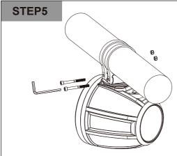
As illustrated, secure the aluminum bands to the metal base using a pair of M6 x 60mm screws, M6 flat washers, and M6 locknuts. The locknuts must be installed into the hex shaped recess on one end of each aluminum band.
