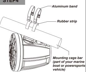
Place a supplied rubber strip around the cage bar to prevent abrasion and secure clamping. Then push two supplied aluminum bands over the cage bar, and align the aluminum bands with the metal base on the speakers.
