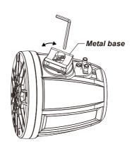
Twist the metal base to determine the optimal mounting angle for the speaker on the cage bar. Then secure the metal base by tightening the two screws.
